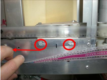
Loosen the 2 screws of the DOW roller 2 turns, push it to the left
