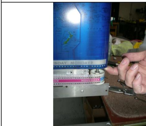
Ensure map is NOT riding in the sprocket of the rear roller by holding the map away with your finger.
