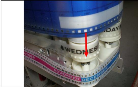
Gently pull the map over the day of week band, aligning the perforations as best as possible. Slide the map perforations over the roller sprocket
